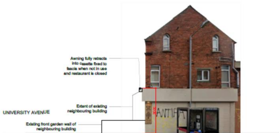
Proposed West Facing Elevation (shown with awning retracted)
