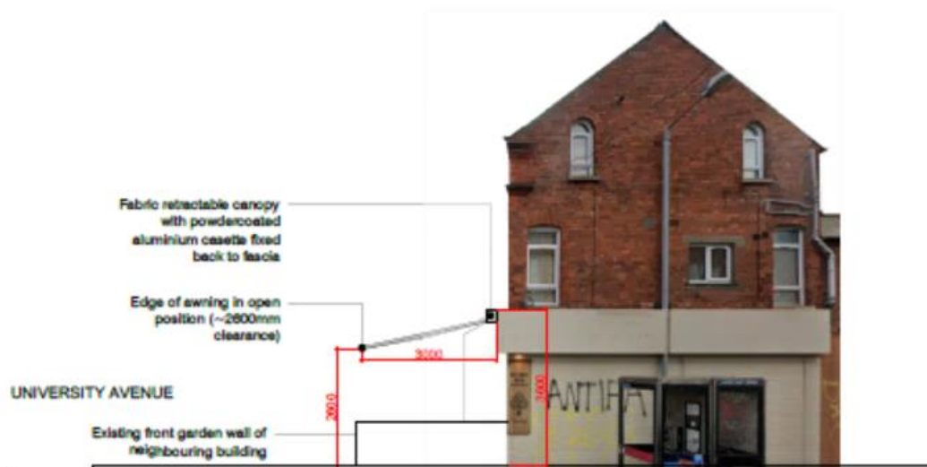
Proposed West Facing Elevation (shown with awning opened)
